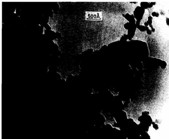
Fig. 6. Electron micrograph showing ruthenium metal particles formed by reduction (at 350 °C in hydrogen) of sample prepared from [H_4Ru_4(CO)_{12}] and TiO_2 .
